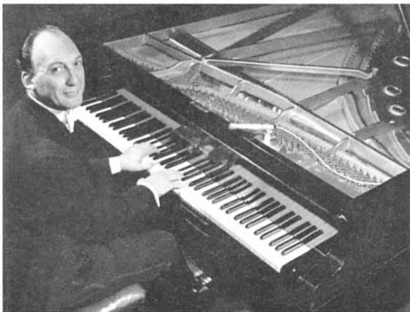
Semprini at the keyboard. A Neumann KM54 condenser microphone is being used here for speech. The polar diagram for this microphone is roughly cardioid—so it will also pick up a fair amount of sound from the piano; and the balance between the two may be satisfactory from the point of view of level. However, the quality of the piano sound will be tolerable only for short periods, and as soon as the "speech-over-music" is finished it will be better to crossfade to a more orthodox balance, if a transition can be made satisfactorily. Also, as it's so easy to pick up vibrations through a microphone stand of this sort, a suspended microphone would be preferred for a sound radio balance
