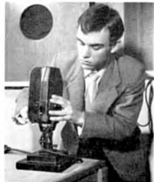
Top: The BBC Portable Effects Unit (or "distort box") for providing filtered speech, used for telephone or P.A. quality, etc., in radio plays. Below: Fixing a baffle to the back of a ribbon microphone.
