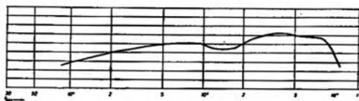
Fig. 4. The frequency response of the AKG D 9
