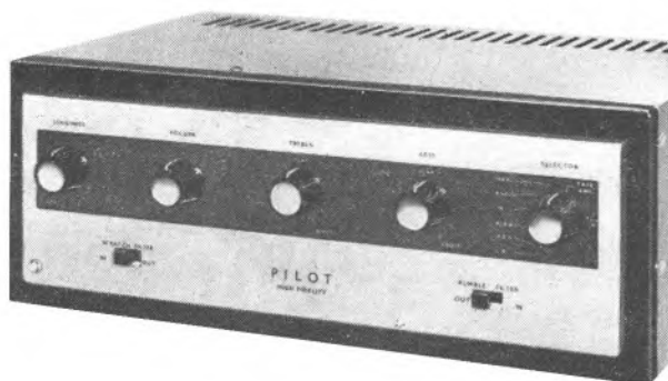
The front panel of the handsome Pilot HFA11 combined amplifier and control unit, showing the seven controls provided
