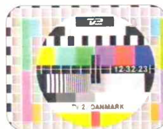
Fig. 4: The PM5534 test card radiated by TV-2 in Denmark.
