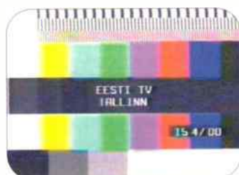
Fig. 2: The Philips PM5537 colour block-board test pattern from Eesti TV in Estonia which includes the identification 'Tallinn'.
