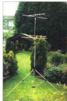
Fig. 4: Temporary mount for crossed-dipole - from Dave Ball.
