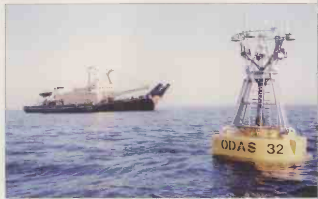
Met. Office ODAS (Ocean Data Acquisition Systems) moored weather buoy. Crown copyright.
