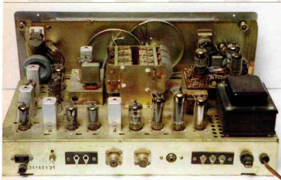
Interior of HE-80 with the p.s.u. on the right, i.f. along left wall, detectors and a.f. output along rear wall. Two metre converter upper right.
