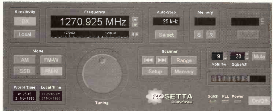
WINRADIO Windows screen showing the representation of a radio receiver front panel on the screen.
