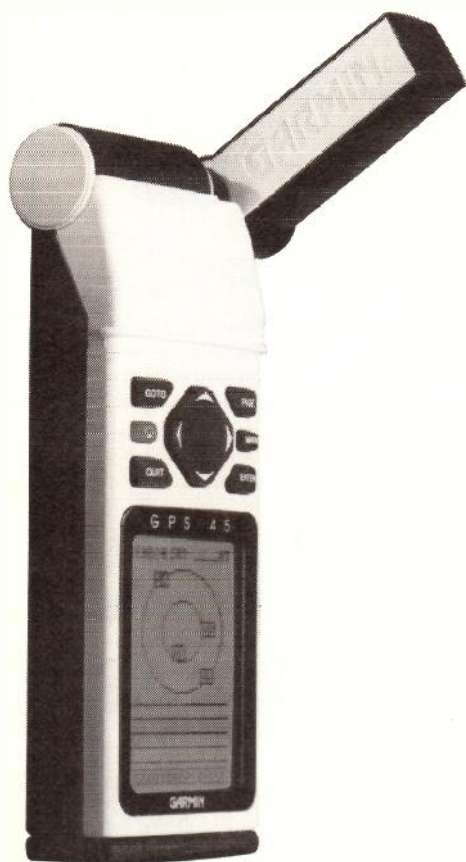
The Garmin GPS 45. The antenna can be removed and connected by coaxial cable to give a better 'view' of the satellites.
