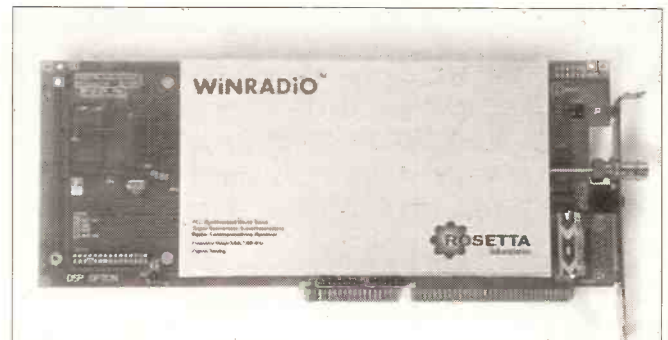
The WINRADIO plug-in card is well screened against r.f. interference from the host computer.
