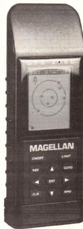
The Magellan GPS 2000 SAT STATUS screen showing the satellites that can be seen by the unit.
