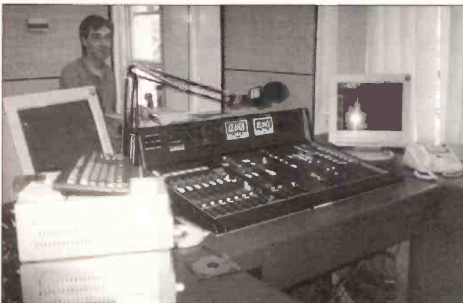
Station Engineer, John Bryans, puts the finishing touches to the new on-air studio, complete with touch sensitive screen and playlist stored entirely in digital form on hard disk.
