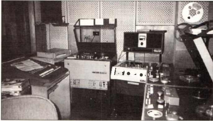
Radio Havana's programming suite showing a Delta mixer-fader unit, an STM-200-k reel-to-reel recording and dubbing unit, and Denon reel-to-reel recorder/playback machines.
