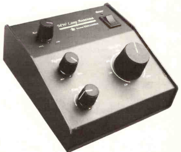
The Control Box is also finished in all-black and contains the power supply and the controls.
