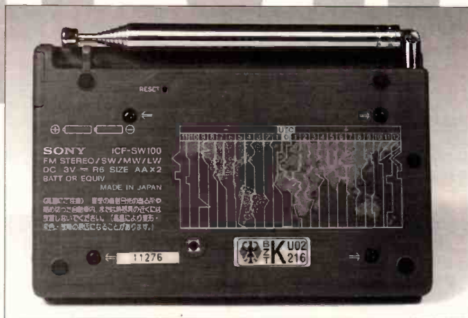
The bottom of the ICF-SW100 carries a variety of information including a world time zone map. The telescopic antenna is shown in its intermediate position.
