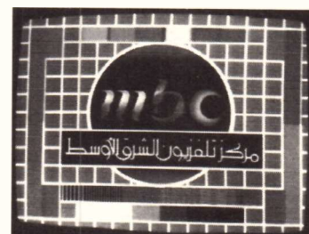
The Middle East Broadcasting test card via Eutelsat II F1 13°E 11.55GHz horizontal received by Peter de Jong using a 900mm dish.
