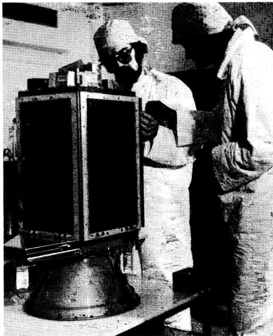
Fig. 1.1: A typical amateur radio satellite, UoSAT-B, in the clean room during construction. Ian Ferebee (left) and Christine Sweeting are members of the University of Surrey Spacecraft team.
