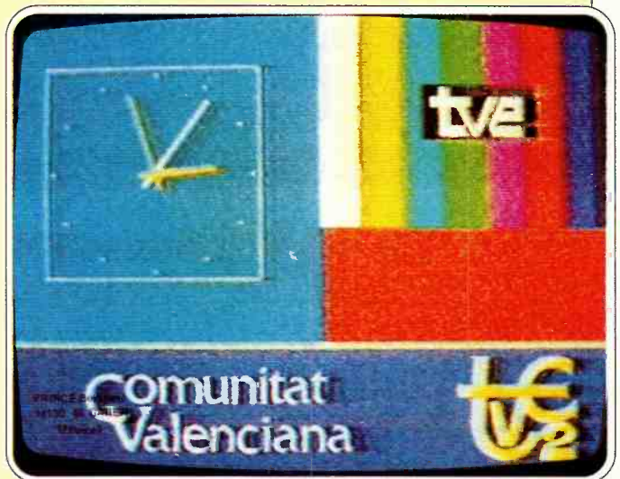
A combined colour-bar test pattern and clock caption used by several TVE-2 regions with suitable local identification.
