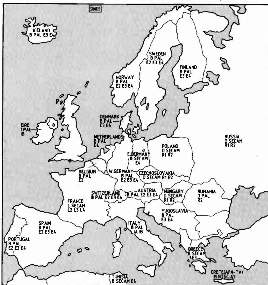
Fig. 1: Map showing transmission standards, colour systems and channels adopted by countries which may be received in the UK. Note that the Austrian channel E2a has the same vision frequency as R1. Also, the Irish channel B shares the same frequency as the Italian channel IA.
