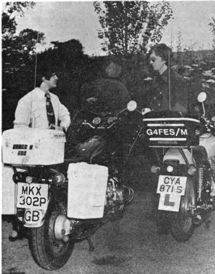
Chris Rycroft, G4FES, is claiming a 'first' with a 2m. FM mobile-to-mobile contact on July 30th with fellow-motorcyclist Bob Smith, G8NCT. Both riders operate semi-permanent installations: G4FES/M uses a Trio TR-2200G transceiver and whip aerial on his Honda CJ250T, while G8NCT runs an Icom IC-240 and whip aerial on his Honda GL1000 "Gold Wing." These two regularly operate mobile on their machines, and this particular QSO was on simplex; they hope 70 cm. mobile will follow before long.
