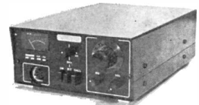
AK20, STE. Latest model from the famous STE Milan range of equipment. 12 channel operation in the 144-146 MHz range. 11-15v. DC operation. 3 watts output. Sensitivity 0.2 uv R.I.T. tone burst. Complete with microphone, and mobile bracket.
