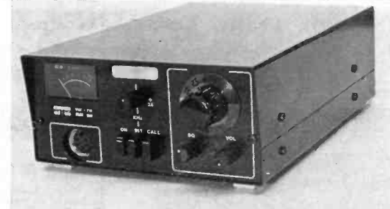
AK20, STE. Latest model from the famous STE Milan range of equipment. 12 channel operation in the 144-146 MHz range. 11-15v. DC operation. 3 watt output. Sensitivity 0.2uv R.I.T. tone burst. Complete with microphone.
