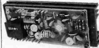
Linear Amplifier. Frequency 144-146 MHz output 10 watts FM, 8 watt PEP SSB. 8 watt AM. Input power 1 watt FM. 25 watt AM. SSB. Input impedance 50 ohm output impedance 50-75 ohm. 12v. DC.
