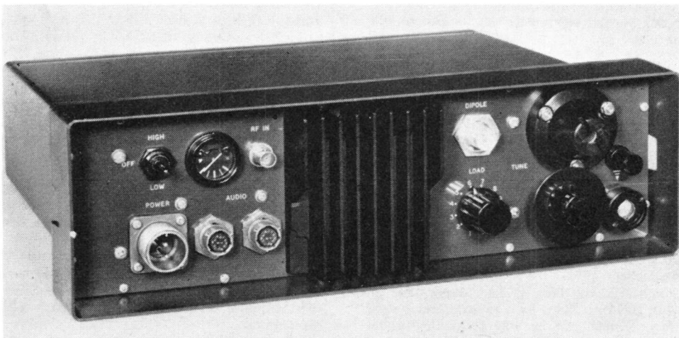
The new Racal TA-944 is a 100-watt linear RF amplifier designed for the range 1.6-30 MHz. It incorporates an ATU which will match the PA into any sort of aerial from an 8ft. whip to 3.0 MHz dipole. It is intended for portable, mobile or fixed-station operation and will give 100 watts p.e.p. output at drive levels of between one watt and 5 watts only.
