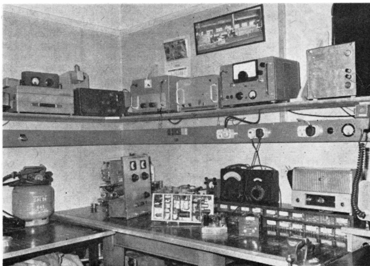
In our May issue, the subject of "The Other Man's Station" feature was G3WVD, Ilkley, Yorkshire. Here we see another part of the G3WVD set-up. Each plug-point is separately switched and fused and there is ample space for experimental and constructional work. He also has plenty of room for aerials, and facilities for an earthing system that should show a very low resistance.
