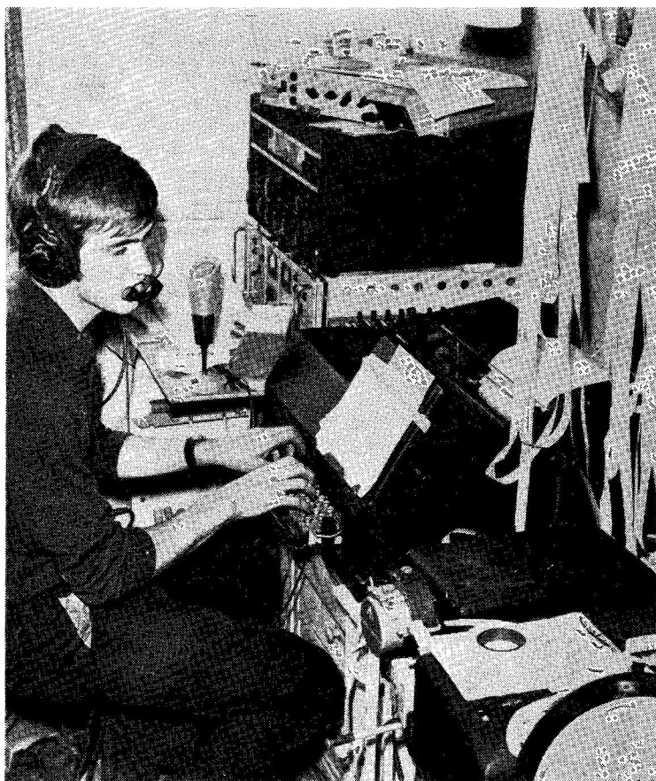
John Liversidge, G8BNW, 54 Boston Road, Horncastle, Lincs. runs RTTY on two metres, his T/P gear being Creed 7B printer, 7TR reperfector and 6S auto-Tx, 850 c/s FSK, at 50 bauds. The on-the-air Tx is 30-watt, into an 8/8 at 45ft., and the Rx an FET converter (to a recent "Magazine" design), with an AR88D. A year's two-metre RTTY activity has so far produced contacts only with G6CW, G8BBB, G8BLG and G8CUO. However, John says that while searching for other 2m. RTTY stations—for whom he is always looking—he gets out quite well on straight two-metre phone.
