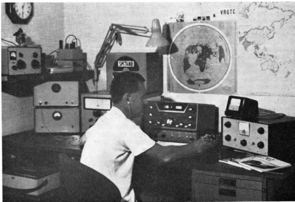
Station of SM7ANB, Lyckeby, Sweden, who runs a 500-watt CW transmitter, and 200w AM phone, all home built. His receiver is a Hallicrafters SX-177 and the aerials available are a 3-element beam, a long-wire and a vertical arrangement for 40 metres. The DX score stands at 299 countries confirmed. Nils is one of Sweden's leading DX operators
