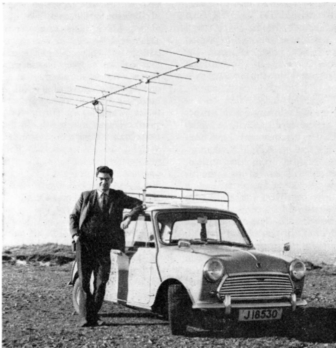
The 8-ele flat-top used by GC8AAZ/P, Jersey, for two-metre operation from high ground in the north of the Island. Change of directivity is obtained by the simple process of turning the car round! The beam assembly breaks down into sections carried in the boot, only the roof-rack and two short uprights being fixtures. Many good cross-Channel contacts have been made by GC8AAZ/P on fine Sunday evenings.
