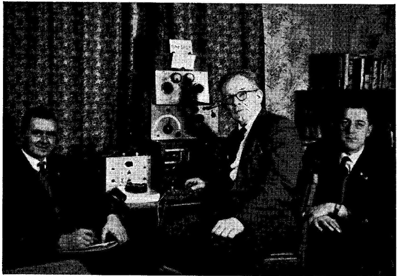
The Welsh team that did so well in the Eighteenth MCC — left to right: GW3KSQ, GW3FSP (call signed for the Port Talbot Club), and GW3BQY. Knocking up 803 points to run into first place, their Tx was a 3-stage gang-tuned job, using screen block keying, with a 3-way foot switch for receive-net-transmit; their Rx was an AR88D, and the aerial a 275-ft. top, 40ft. high and well in the clear, running near enough N-S, and Zepp-fed through 66-ft. feeders. Their operating throughout was first rate — as the results show, it was that and not the scoring system that brought them out on top. Well done, boys—back!
