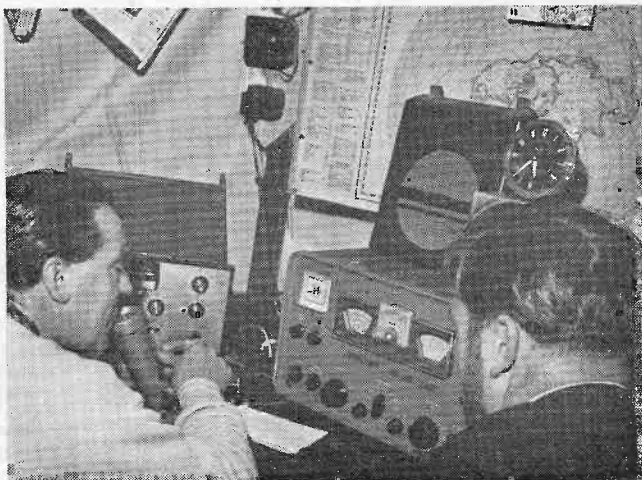
When the Stroud & District Radio Club organised their public appearance at the annual show locally, this was the set-up. Under the callsign G3SDR/A, operation was mainly on 20-metre Side-band, using a linear amplifier consisting of four 807's to get 300w. p.e.p., with a Hammarlund HQ-170 as receiver. The beam in this picture is a Mosley Tri-Bander, and at the controls when G3GMN took the photograph was G3GEW (at left).
