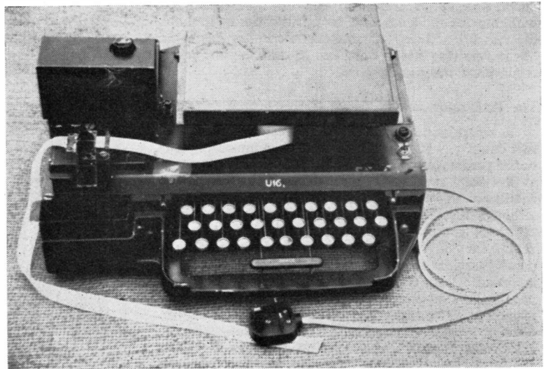
General appearance of the Perforator Model 44, Mk. II. This machine punches tape, enabling a message to be set up prior to transmission, and uneven or uncertain keyboard operation avoided under actual transmitting conditions. Details are discussed in the text.
