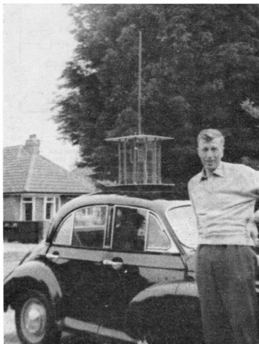
When G2HKU/M (Sheerness) visited his old friend G6AB (Holland-on-Sea, Essex) and a well-known callsign on Top Band, the latter decided that what G2HKU really needed was a proper loading coil designed on the principles of utmost RF efficiency and highest-Q, to 1930 standards. The thing came out to be about 12 times larger than the Tx and, as it also constituted a built-in head-wind for G2HKU's car, it was found impracticable to use it on the road — but it does work!
