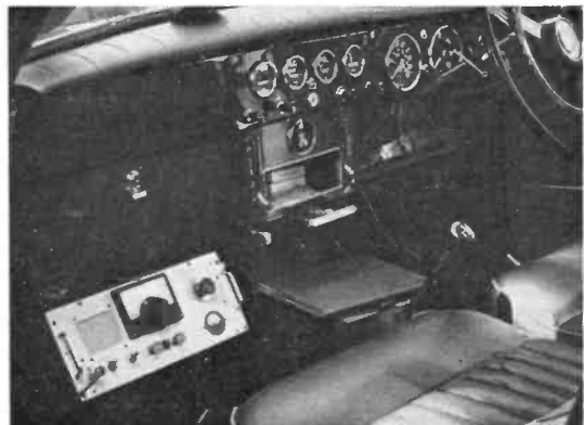
A good example of a two-metre mobile transceiver installation, seen at one of the recent rallies. Fitted on the passenger side, it still leaves ample leg-room.
