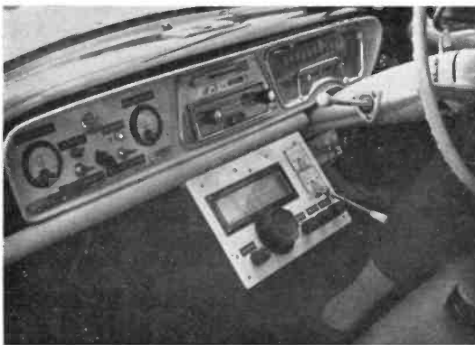
G3FUR (Stamford) has a particularly impressive two-metre mobile Tx/Rx, installed in his Simca. The lever is for change-over control (just a flick), and the panel in the glove compartment on the left is for main switching and auxiliary charging.
