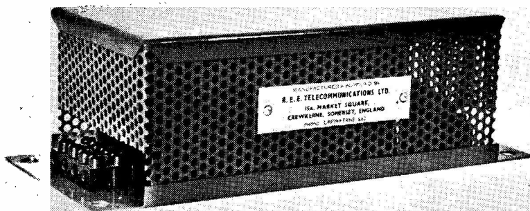
The new Telecomm 40-watt transistorised DC converter, specially developed for use with mobile/portable gear. It will provide a compact, silent and efficient source of DC power at 300v. 130 mA from a 12-volt car battery.
