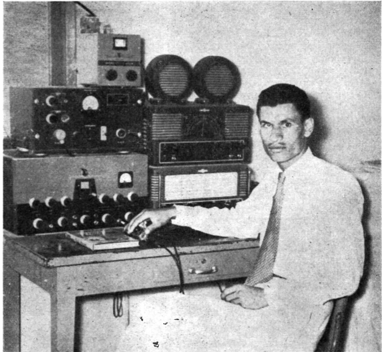
MP4KDS, at Kuwait, Persian Gulf, is ex-OD5BM; he runs 100w. to an American Viking transmitter, his receiver being an Eddystone 840A. The aerial is a three-element rotary beam.
