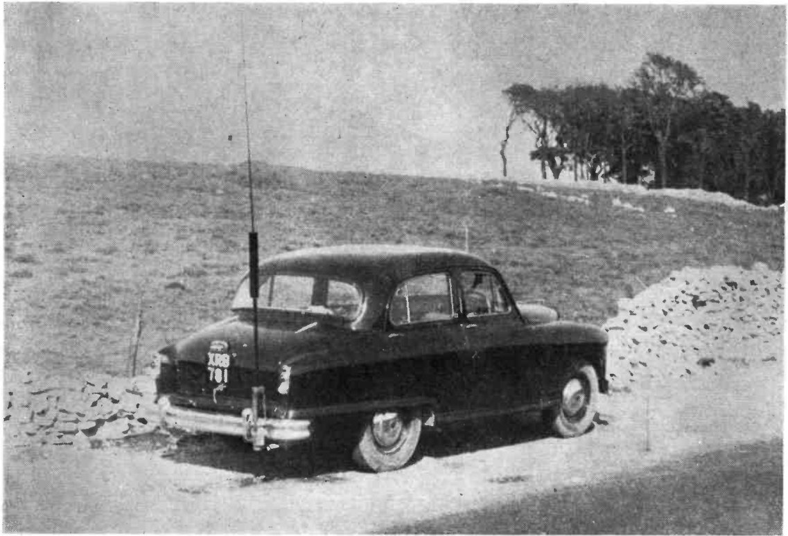
This photograph gives a very good idea of the aerial arrangement used by G5CP, and its scale. The loading coil is the cylindrical fitting on the whip, and notes on the construction of this coil and the adjustment of the aerial itself are given in the text. The car is a Vanguard, and the equipment used is a ZCI Mk. II (carried in the boot) modified as described in the article. G5CP/M can be heard on about 1900 kc.
