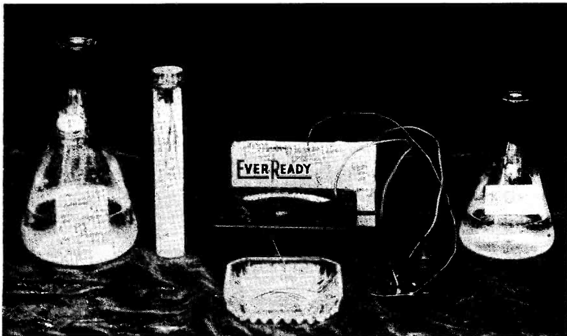
Equipment and set-up for pointing the whiskers—see Fig. 2 for circuit. Also shown are flasks of caustic potash solution (KOH) and distilled water. The test tube is used for storing whiskers to protect the points after processing. In the foreground is the pan in which the points are formed by electrolytic action, as described in the text.
