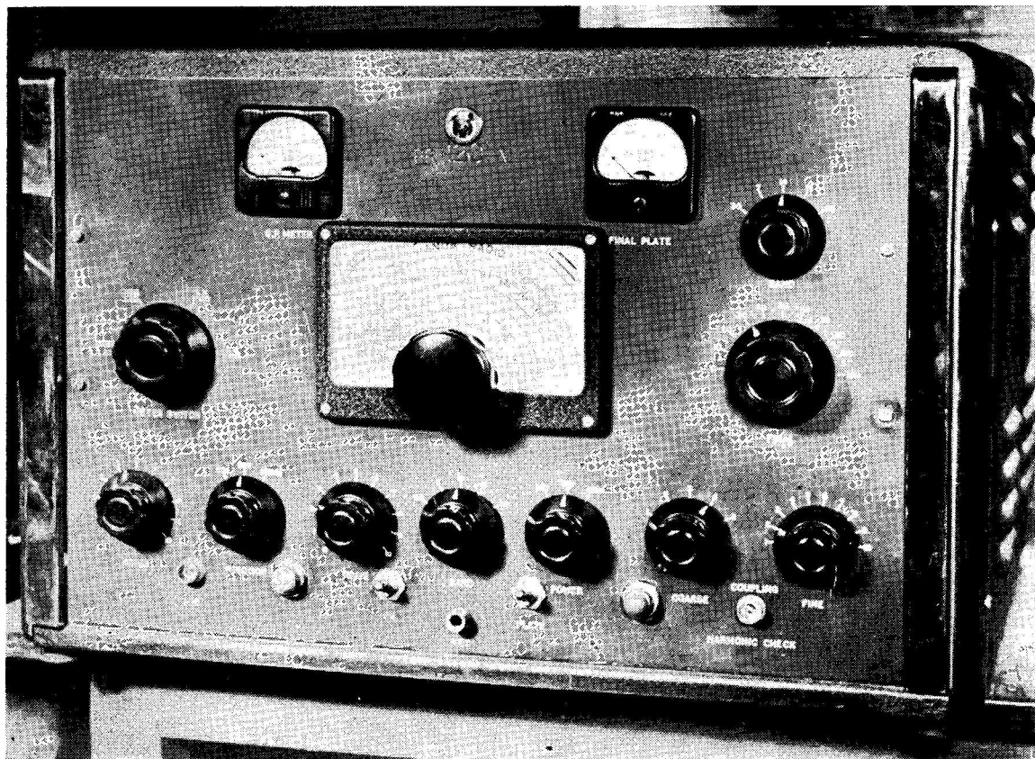
Front panel appearance of the Panda PR-120-V, which is self-contained for CW/Phone operation on all bands 28-3.5 mc, is fully TVI-proofed, and fitted with an exceptionally stable VFO. Most of the controls can be identified in this photograph.
