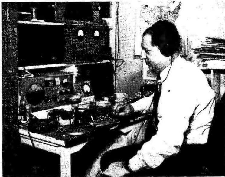
Station of ZS6ACD, Johannesburg, who does not consider himself DX to G's! His transmitter is VFO 6V6-6L6-807 running 50 watts, and the receiver is an SX-43. Aerials are folded dipoles, made of 300 ohm ribbon, for Twenty and Forty. ZS6ACD is very badly situated in terms of local interference.
