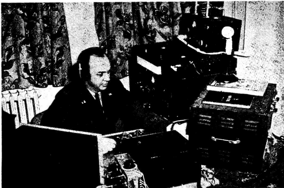
"My station and I," as DL4EF (Frankfurt) puts it. The Tx is a modified BC-610, with a Meissner Signal Shifter (the original pre-war conception of what we now call a VFO) and the receiver is a Super-Pro. Captain Hamel has been on the air since 1919, and was at one time VO6T, Goose Bay, Labrador. His home call is W3ORO, at Silver Hill, Maryland.
