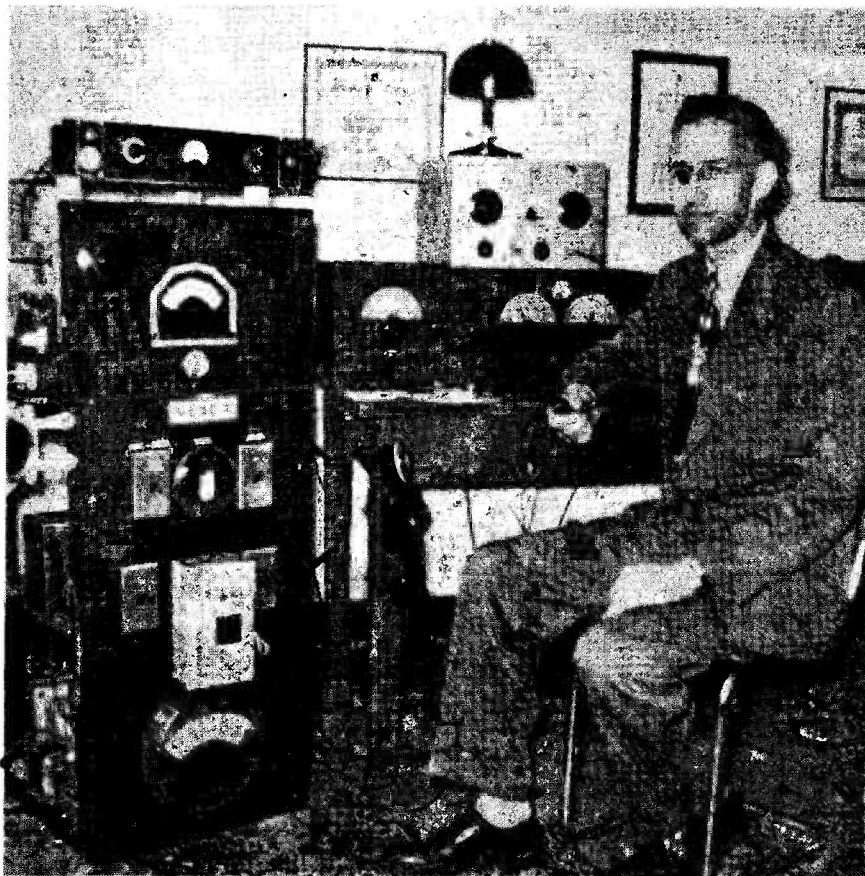
VE1EA, Windsor, Nova Scotia, "right on the edge of the ocean," is well known as a consistent signal when it comes to Top Band DX. His receiver is an RME-69 with DB-20 preselector and his station a good example of neat, individual design.
