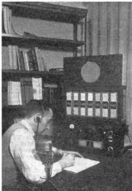
ON4AD, Ghent, Belgium, runs this nice-looking outfit on 3.5, 7, 14 and 28 mc. The PA is an 813, modulated by four 807's in parallel push-pull. The receiver is an HRO. Everything on the transmitter side—VFO, driver, PA, speech amplifier, modulator and power packs—is carried on the rack assembly.
