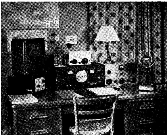
HB9BZ, Uster, Zurich, has a 5- and 6-metre converter into his SX-17. On the right of the receiver is the all-band transmitter, using an 815 in the final and running up to 35-40 watts on CW and 'phone
