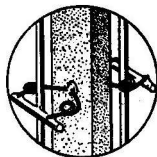
V Wire Mounting British Patent No. 578290
