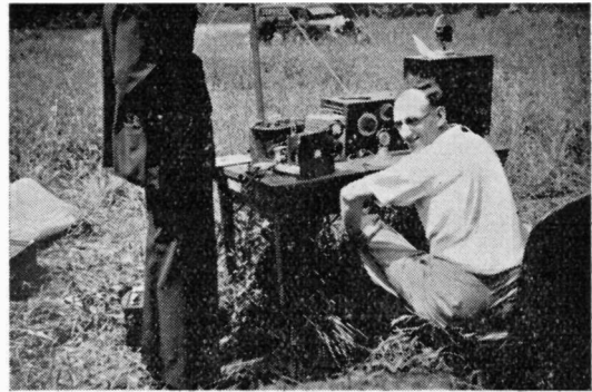
G2UXP, Westerham Hill. The very compact TX. (6C5 CO-6L6 PA-6C5/6L6 mod.) is on the corner of the table, with G4DC at the microphone. The RX and F/S meter are to recent "Short-Wave Magazine" design.
