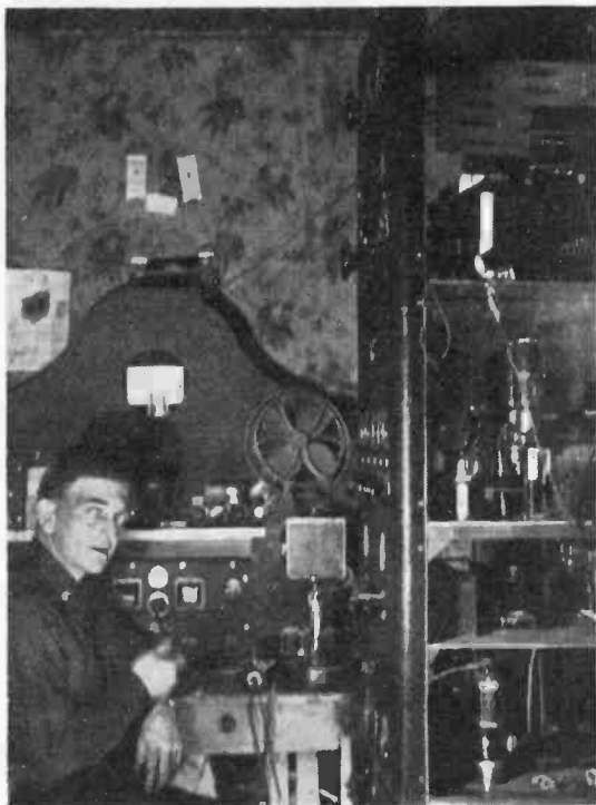
Operating position and equipment at W2JZR. The final is a pair of 204A's drawing 950 watts and giving a measured RF output of 837 watts. Quite a nice lot, even for 1.7 Mc.
