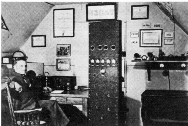
General view of W2CAY, Albert Dabb, at Linden, New Jersey. He was well heard and worked G2PL and G2DQ. The 1.7/3.5 Mc rig is on the shelf to the right, with a 203A in the final and 200 watts input.
