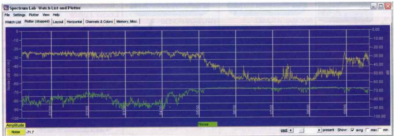
● Fig. 10: Spectrum Laboratory can automatically measure and plot signal levels as well as background atmospheric noise. Here, the yellow line shows signal strength of Canadian time signal station CHU on 14.670MHz, and the green line is the noise level. The difference between them - the signal-to-noise ratio - is an indication of reception quality.
