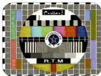
● Fig. 2: The Moroccan PM5544 test card with a distinctive modification to the centre.
