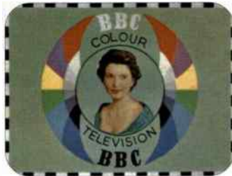
● Fig. 3: The BBC Colour Tuning Signal radiated during 405-line NTSC test transmissions in 1956.
