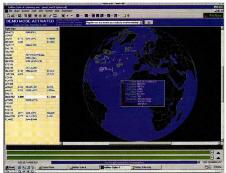
● The Airnav program can also be used to monitor aircraft around the world, shown here displaying a saved log of several aircraft over the Atlantic heading east.
