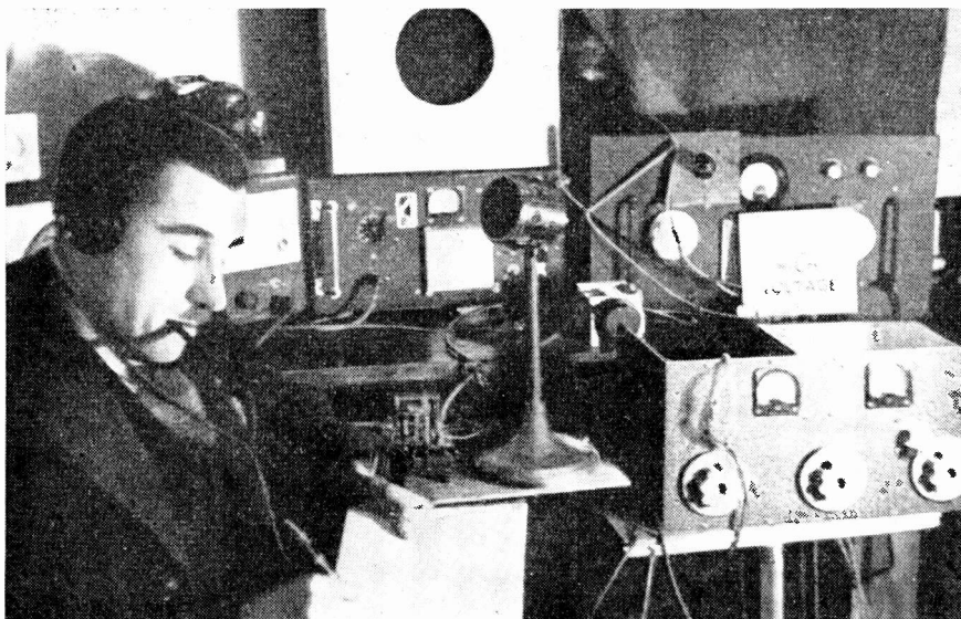
The station of EI4X, Clontarf, Dublin, a keen CW man on the 10-, 20- and 40-metre bands, with phone operation on Forty thrown in. The Tx is VFO-TU5B-807-813, run at 100/150 watts, the Rx an S.40 and the aerial a 67-ft. Zepp.
