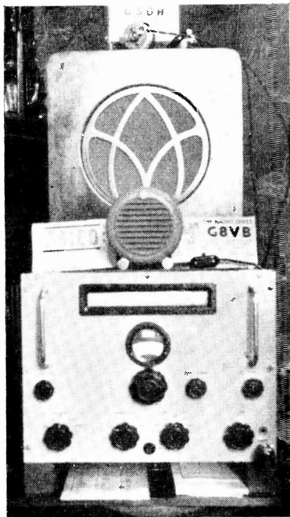
SWL W. G. Johnson, Thornton Heath, Surrey, has a neat outfit, of which the central piece is the CR-100, tuning 10-5000 metres. W. G. J. has this receiver on a turntable, so mounted for the convenience of armchair operation.
