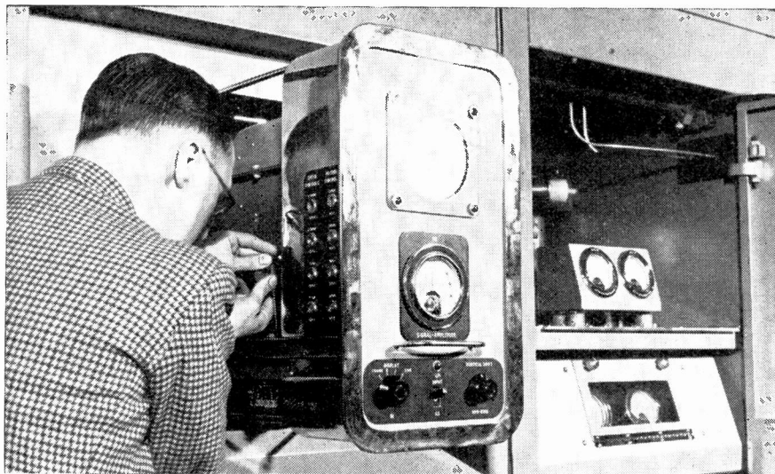
Close-up of the waveform monitor at the BBC's Sutton Coldfield TV transmitting station.
