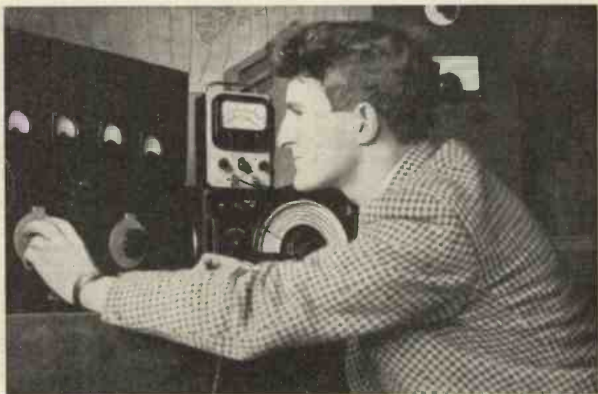
G3BFC, of Ferndown, Dorset, on 7 and 14 mc with CW ; he uses an R.1155 receiver. A full description of the station will be appearing in the "Short Wave Magazine."
