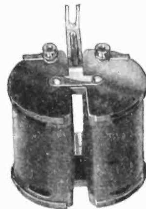
Fig. E. A Binocular coil of unique construction. It is used in self-neutralized type of receivers where oscillations or "squeals" are not desired.
