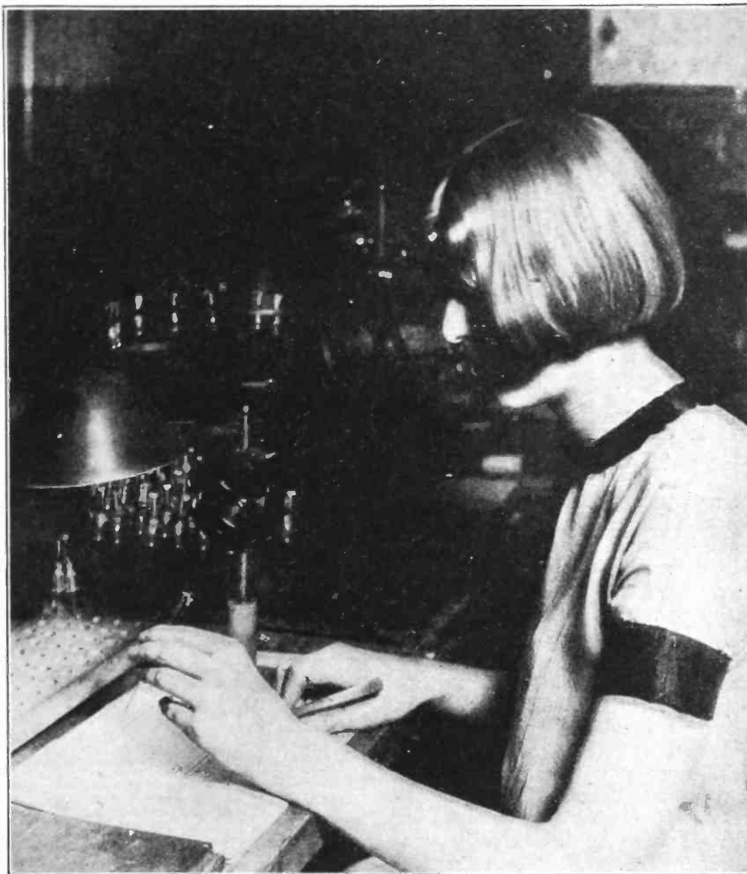
This girl is a check inspector, which means that she checks up the inspections of other inspectors. In her hand is the complete "mount" or inside assembly of a UV-199 tube, with filament, grid, plate, supports, anchorages, flare tube and exhaust tube, ready for insertion in the glass bulb. To ensure the highest standards at all times, the check inspectors take a certain percentage of the parts, in this case the mounts, and give them an extra inspection. A powerful magnifying glass is required to inspect the delicate assembly.
