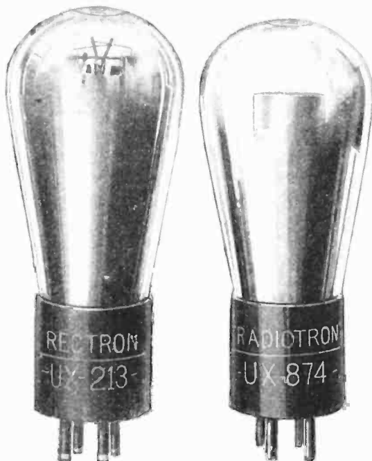
Above shows the UX-213 full wave rectifier tube and the UX-874 voltage regulator as used in power units.
