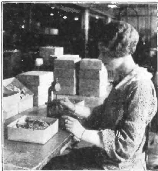
Among the various components supplied to the Radiotron factory are the plates. Here is a girl inspector, testing the plates one by one with a direct-reading micrometer size gauge.
