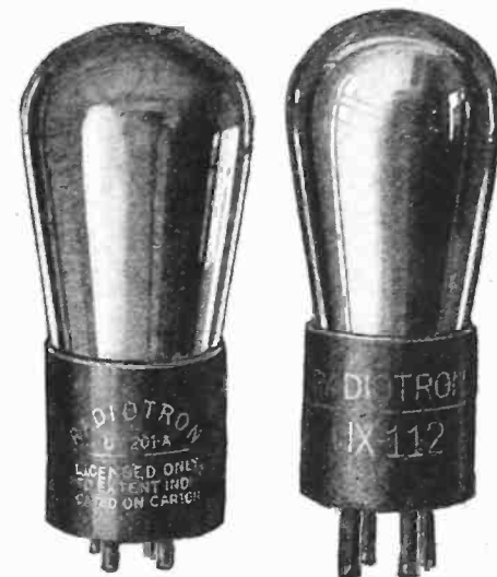
A UV-201-A tube is shown at the left and the new UX-112 power tube at the right.
