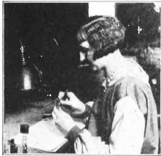
Here are the type UV-201-A tube mounts or inside assembly receiving the regular inspection. The inspector carefully examines each mount, to make certain that there are no mechanical defects. Her sole tool for this work is a pair of delicate tweezers, for this work is of the most delicate kind.
