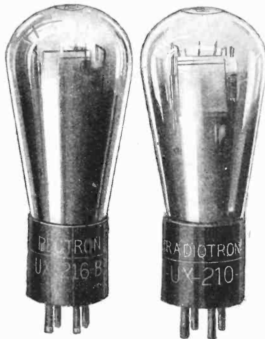
The UX-216-B is commonly used as a half-wave rectifier in power units. The UX-210 at the right is a super power amplifier for use on 8 volt filament supply.
