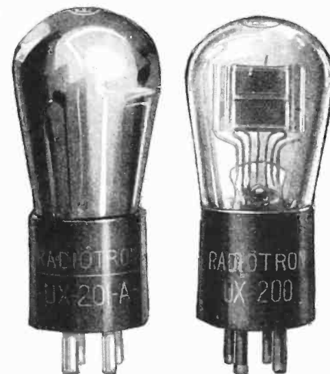
The UX-201-A and the UX-200, the latter type being the most efficient detector.
