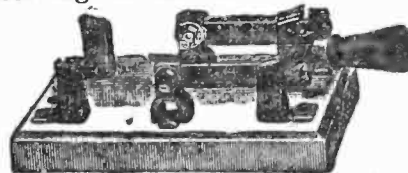
Fig. 1. A simple Aerial Switch
