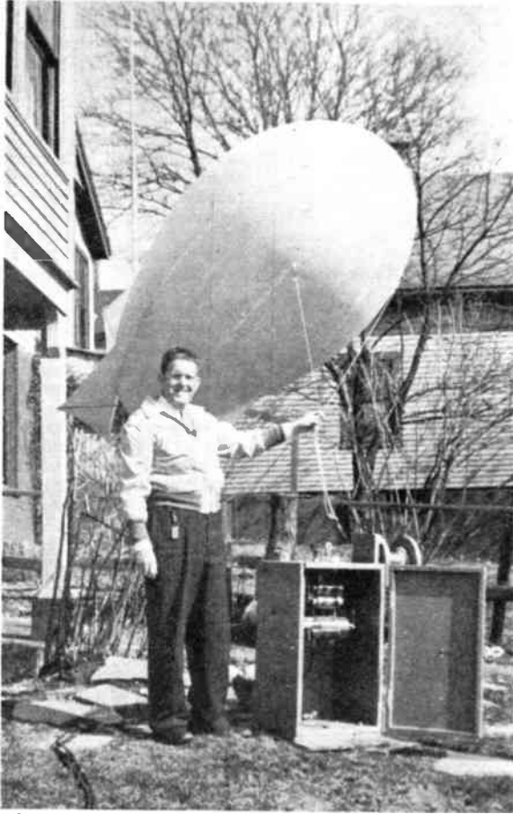
Amateurs are ever resourceful. To get good radiation characteristics when transmitting on the 160-metre band, it is desirable to have an aerial as high and as long as possible. W1BB of Winthrop, Mass., U.S.A. lets his up on a kite-balloon (termed a "Kytoon") and in this photograph we see him with the winch gear and the radio-frequency matching and coupling unit in its weatherproof housing.
