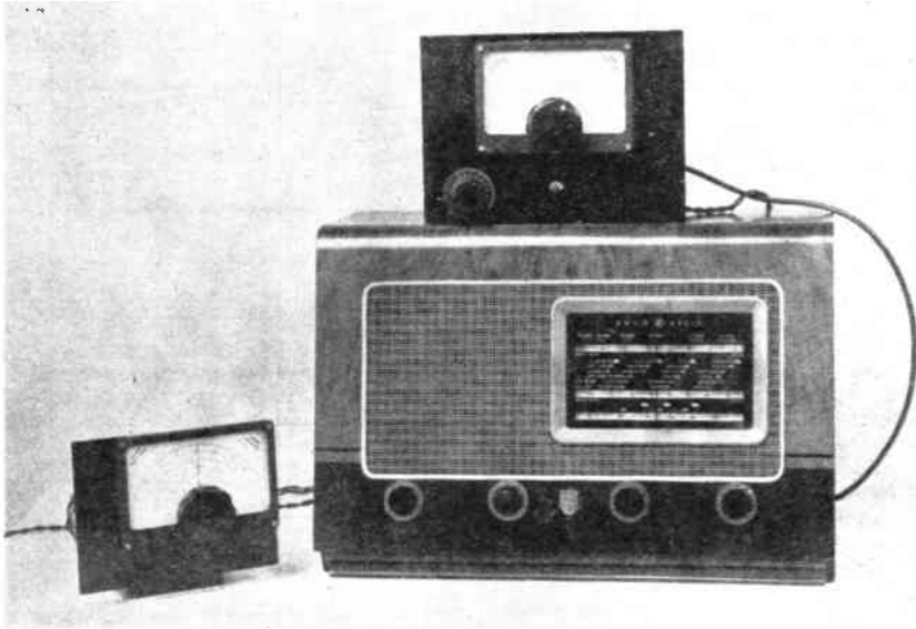
In this photograph, an Ecko A.144 broadcast receiver is shown with the HFM/BFO on the left (the instrument on the receiver is the HF/VHF Converter described in another article in this issue). Full details for the operation of the HFM/BFO with any such BC receiver are given in the text.
