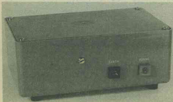
Two sockets, for aerial and earth, are mounted on the rear panel of the case.
