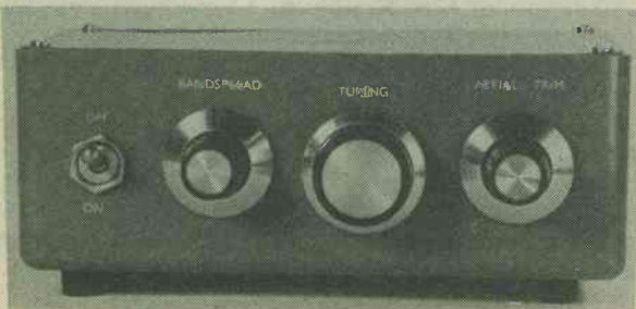
The front panel components, from left to right, are on-off switch S1, VC3, the 2-gang capacitor and VC4.
