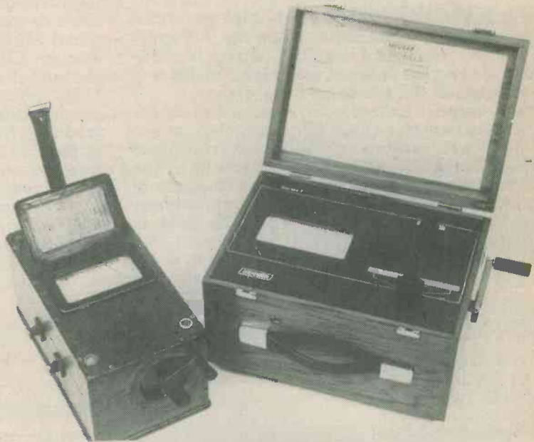
A 1978 MEGGER Model SL2, Series 1 insulation tester alongside one of the self-contained 500V resistance testers of 1904 design. Both use the Evershed cross-coils movement
