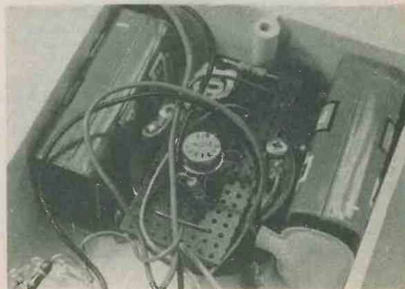
A close-up view of the Veroboard assembly. There are two PP9 batteries, one on either side of the meter
