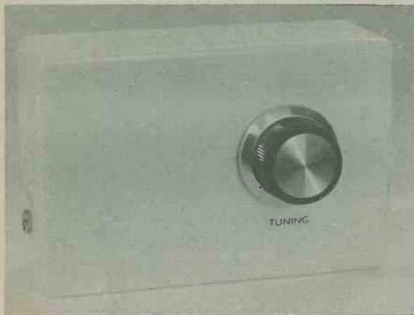
This photograph of the receiver shows the earphone socket mounted on the case side opposite the on-off switch
