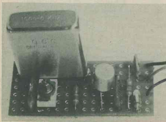
The crystal marker components make up a tidy assembly on the board
