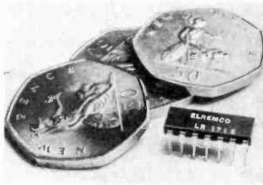
The Eremco LR171E dual-in-line integrated circuit. This functions as a comprehensive timing device, offering timing periods from 5 milliseconds up to 4,000 hours
