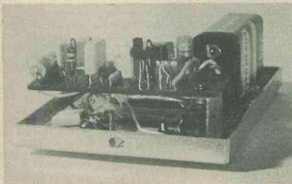
Side view of the Veroboard. Its supporting bracket is secured to the front panel under the body of the key jack socket
